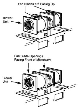
7. Guide wires into duct while placing blower unit back into opening.
